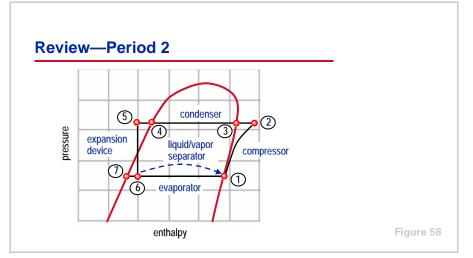
In Period 2, the refrigeration cycle of the helical-rotary water chiller was examined on a pressure-enthalpy chart. Also, the performance characteristics of the various refrigerants were compared.
